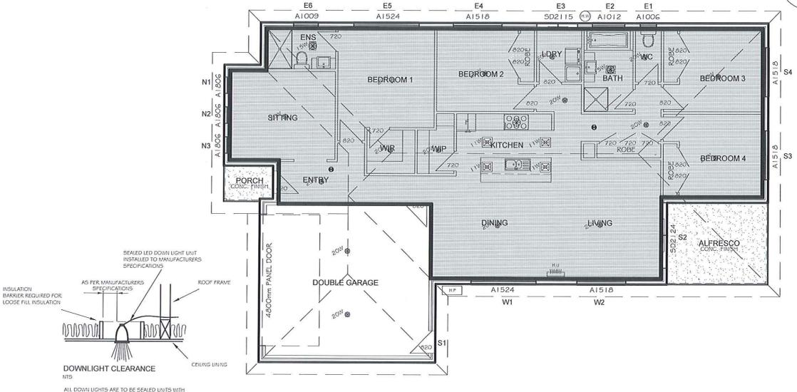
APPROVED INSULATION BARRIERS. ( SEALED TO PREVENT AIR LEAKAGE FROM LIVING ZONES INTO ROOF SPACE ). IF VENTED DOWN LIGHTS ARE USED THE ENERGY REPORT WILL REQUIRE AMENDMENT. ALL LIGHTING IS TO BE INSTALLED STRICTLY IN ACCORDANCE WITH AS3000 AND THE MANUFACTURERS REQUIREMENTS.
